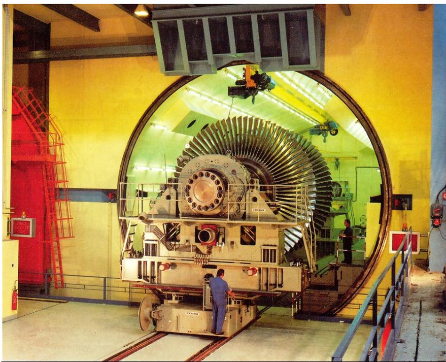
Factory based Overspeed Balancing and Integrity Testing Facility
