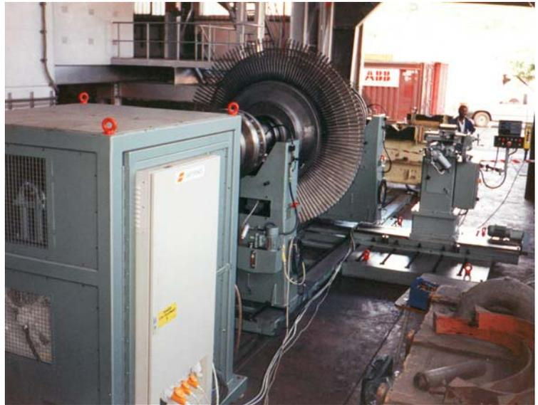
Transportable Balancing Machine with Machining Attachment being used as part of a major overhaul of Turbines in a Power Station in Zimbabwe
