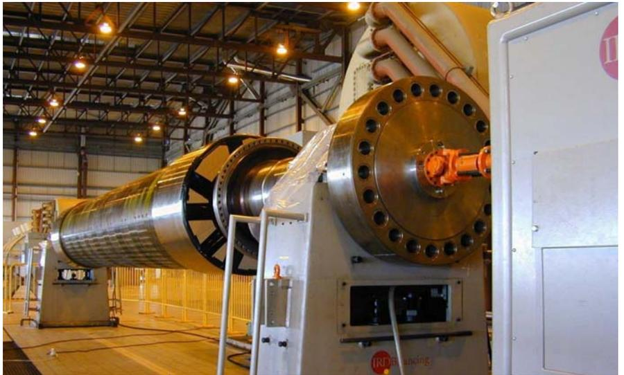
Machining and final balancing of a “Flexible”, 83 tonne Generator Rotor on the suspended floor, alongside the Turbine / Generator Set in a Power Plant
