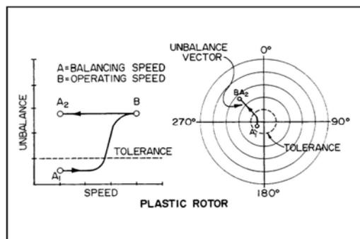
Typical variation of unbalance amount & phase angle relative to changes in speed for a plastic rotor
