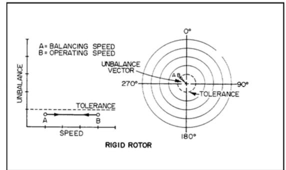
Typical variation of unbalance amount & phase angle relative to changes in speed for a rigid rotor
