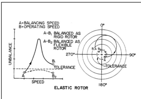
Typical variation of unbalance amount & phase angle of an elastic rotor as it runs up through its first critical speed
