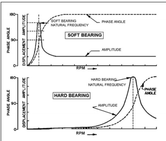
Comparing Amplitude/Speed Response of Hard & Soft Bearing Balancing Machines
