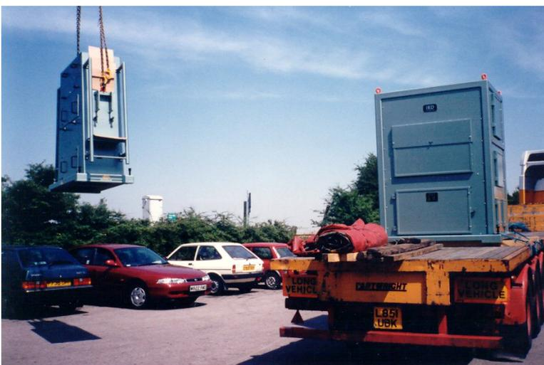
Loading the End Drive Unit and pair of Pedestals of a 100 tonne capacity Balancing Machine System for transporting to the next work site
