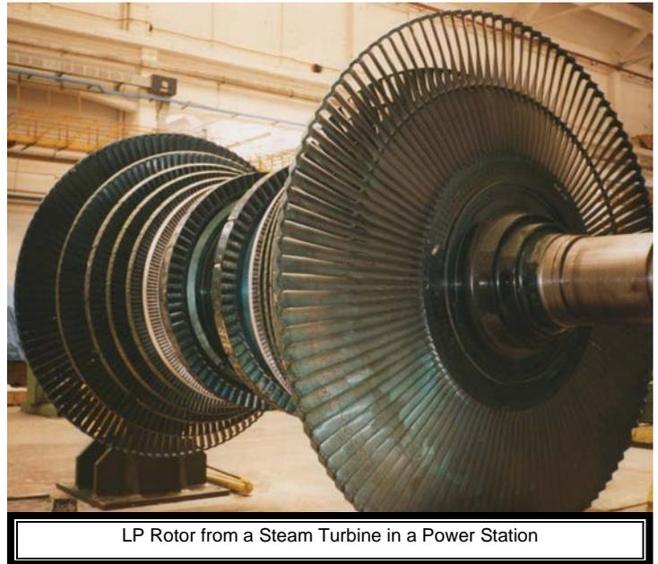
LP Rotor from a Steam Turbine in a Power Station
