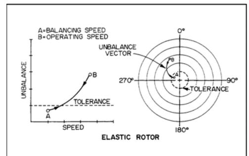
Typical variation of unbalance amount & phase angle relative to changes in speed for an elastic rotor
