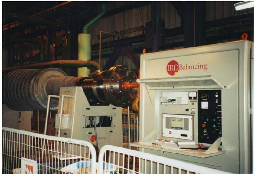
100 tonne capacity Balancing Machine set up on the Ground floor of a Power Plant for balancing an HP Rotor from a Turbine/Generator Set on the 4<sup>th</sup> Floor
