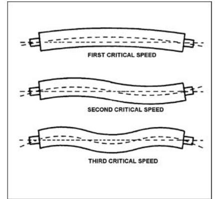
Typical flexural modes of a cylindrical rotor
